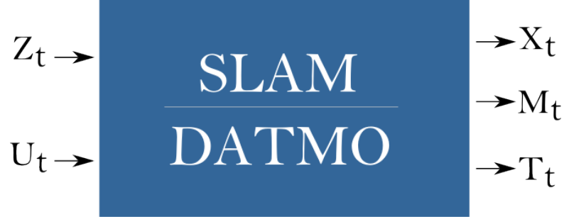
Figure 2.1: Process diagram for intelligent vehicle perception.
